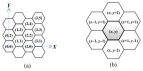
Figure 1: Coordinate system of cellular-based management.(a) Each cell has a unique ID in *CBM* system.(b) Coordinate system of *CBM* is defined.
